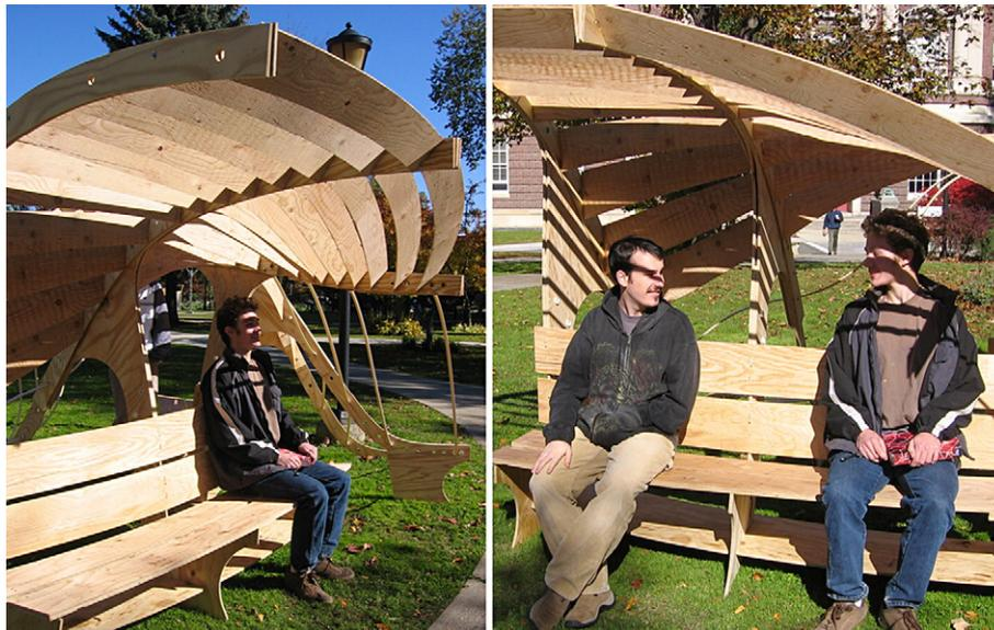
Fig. 2. Sunlight penetrates the louvers of this architectural studio project in an unanticipated way, causing discomfort. An interactive daylight renderer could have predicted this problem, allowing the designer to optimize the orientation of the louvers.
